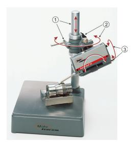
that the bracket with the Pocket Surf unit is tilted, using adjustment ②, to align with the tapered workpiece surface being measured.
