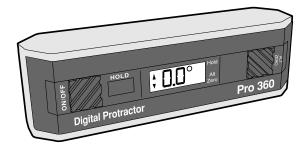
The Pro 360 uses an innovative liquid filled angle sensor. As the protractor is moved, the liquid seeks a new position, resulting in changes in the electrical properties of the sensor. A microprocessor analyzes the changes and calculates the numbers seen on the display.
